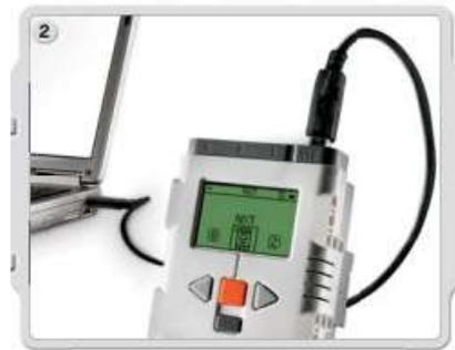
b) Open LabVIEW 2013 program on your computer. Click on “Tools >> NXT/EV3 Terminal..” and verify NXT robot connection.
